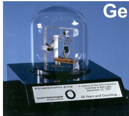
First transistor John Bardeen, William Shockley and Walter Brattain at Bell Labs, 1948
